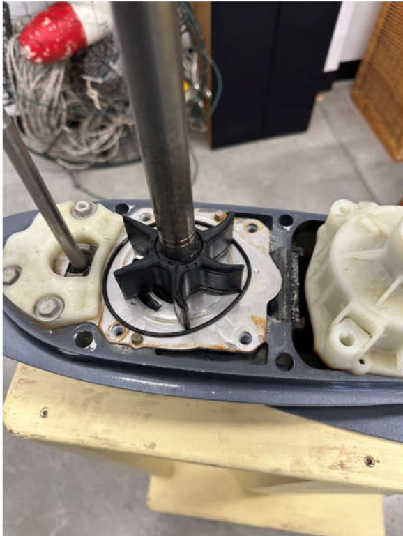
Servicing the water pump
